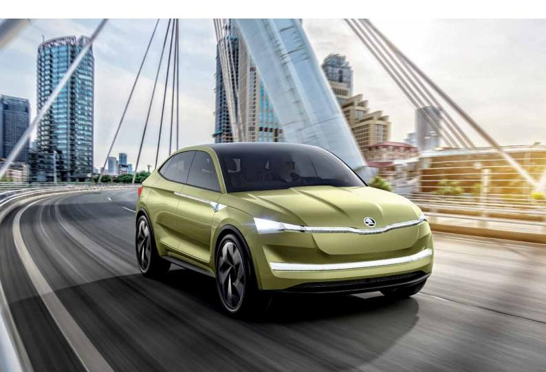
The ŠKODA VISION E study, based on the Group's MEB modular kit for electric vehicles, has a system capacity of 225 kW. Two powerful electric motors enable the car to reach a top speed of 180 km/h. It draws on economical and powerful lithium-ion batteries and smart recuperation, which in practice equates to a range of up to 500 km per charge. The study also entertains the possibility of inductive charging batteries, fast charging to give an 80% charge in 30 minutes, and autonomous driving.
